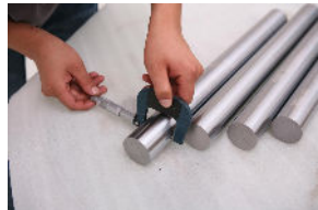
Piston rod outer diameter detection
